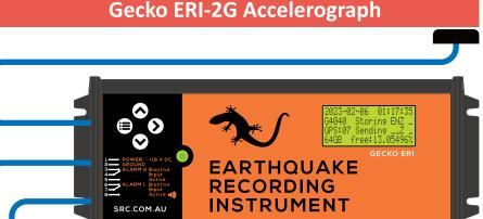
This building monitoring solution comprises a triaxial LCA-2G accelerometer with 2m cable connected to a wall-mountable Gecko earthquake recorder, which includes an Ethernet port, an internal battery for over 12 hours of operation\* in case of loss of AC power, an alarm buzzer, and two switched alarm relays
